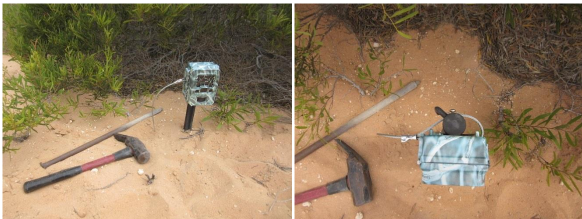
Figure 6. Simple cable and ground anchor used to deter camera theft on Dirk Hartog Island.
