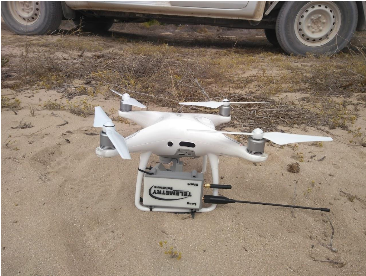
Figure 8. Phantom 4 Pro remotely piloted aircraft (RPA or 'drone') showing attachment of Telemetry Solutions remote-download base-station using cable ties (© S. Cowen/DBCA).
