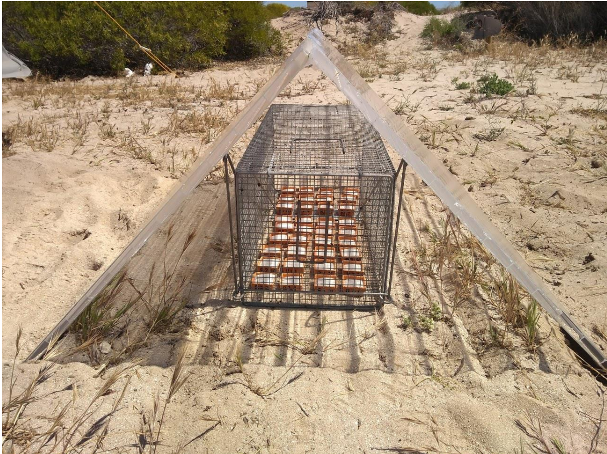
Figure 12. Example of faecal DNA degradation ‘in-situ’ trial set-up, showing Plexiglas ‘A-frame’ and cage-trap with ceramic dishes containing clean, dry sand (© S. Cowen/DBCA).
