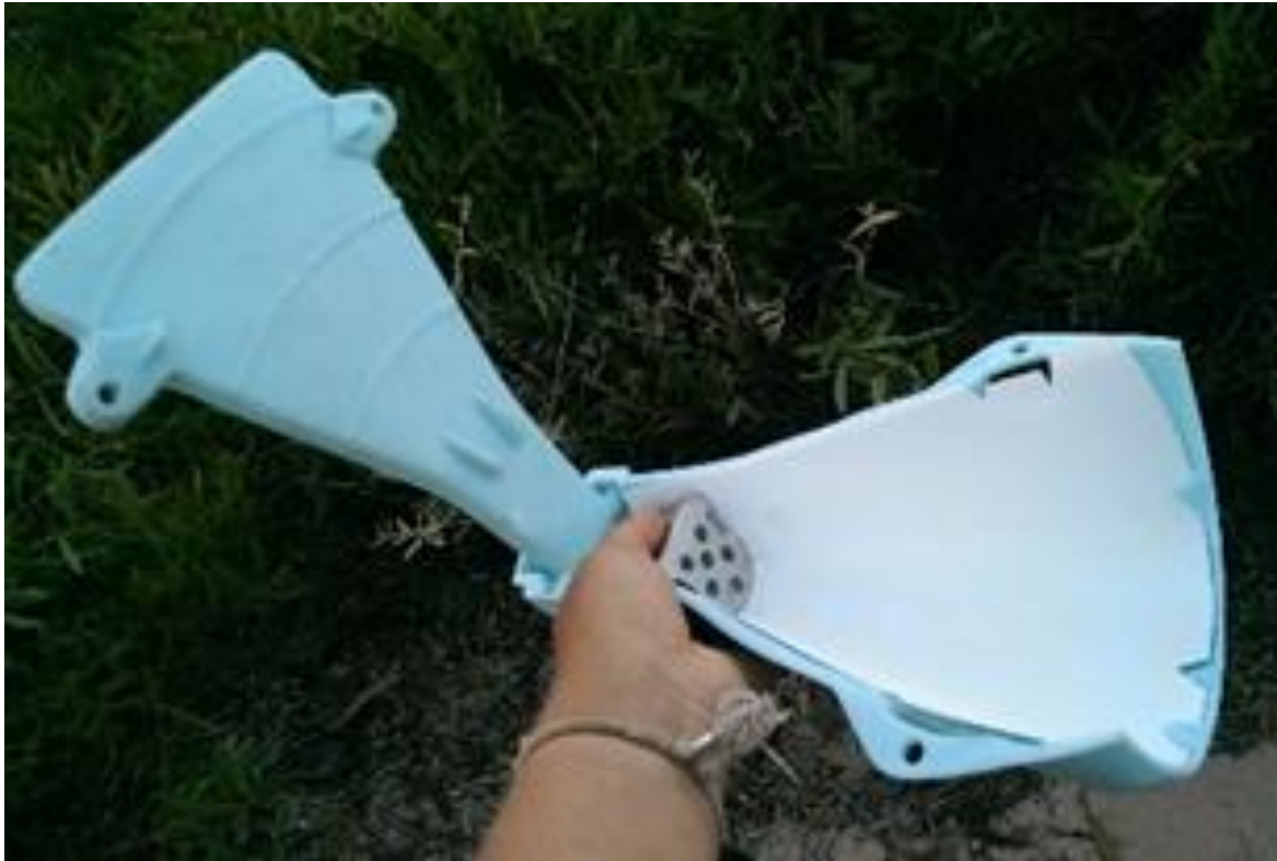
Figure 11. Open hair-funnel showing base with peg-holes for attachment to ground (left), metal chamber for lures (centre) and funnel itself with fresh adhesive wafer (right) (© L. Scheelen/DBCA).
