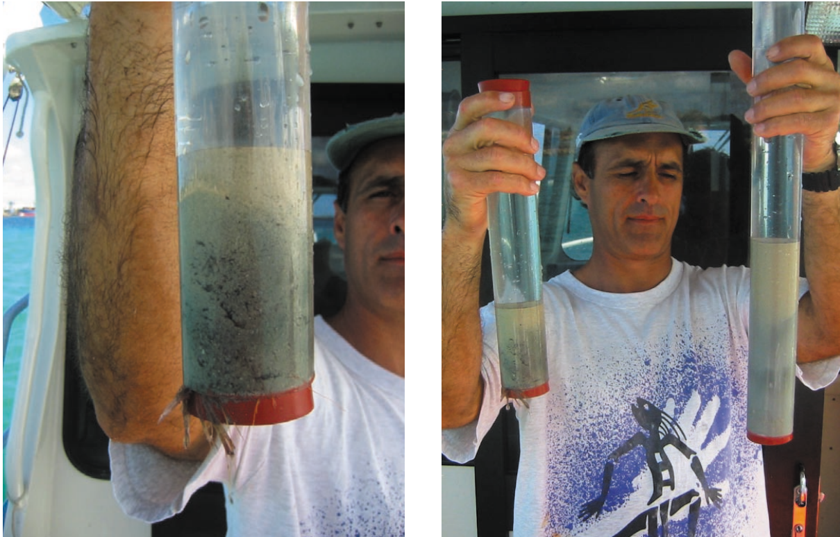
Figure 3: Sediment cores taken from site CB1 showing the white fine grained sediment overlaying the original coarser grained grey sediments and decomposing seagrass rhizome.
