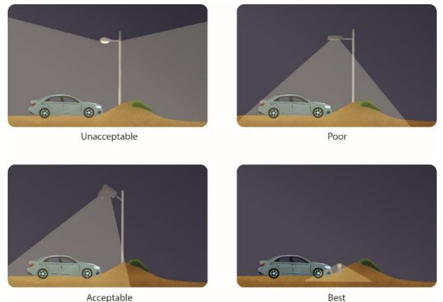
Figure 14 Lighting options for a parking area. Figure adapted from Witherington and Martin (2003) 3 .
