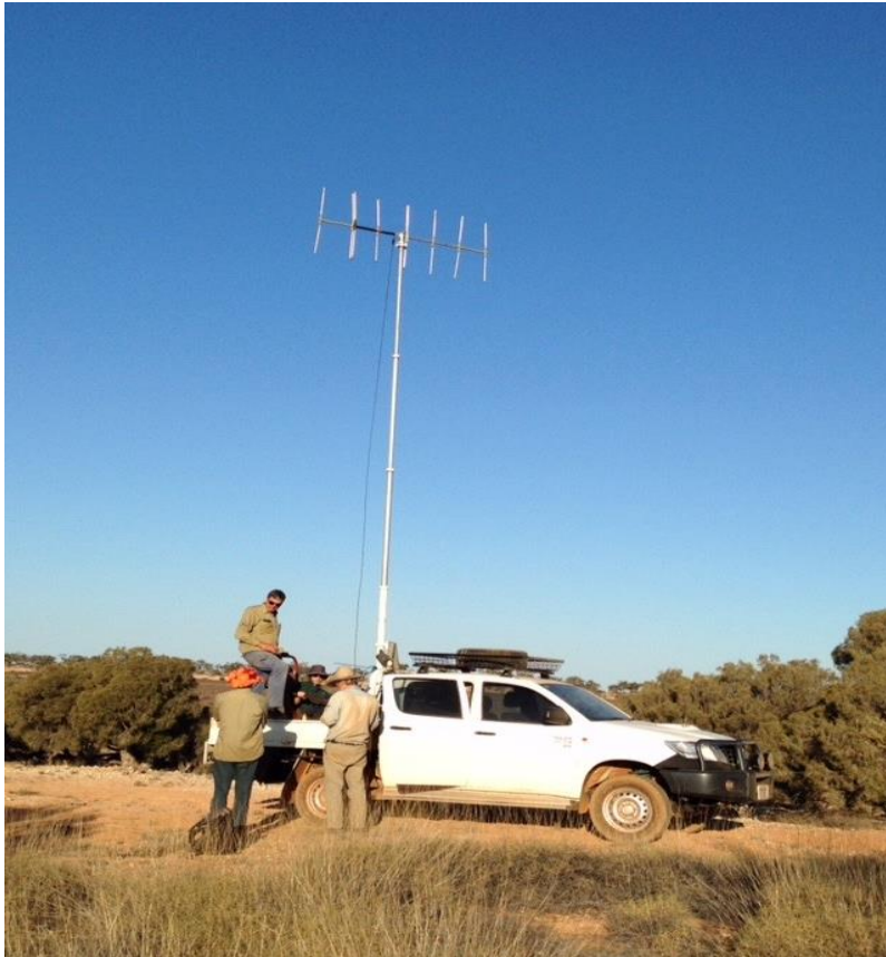
Figure 3. Adrian Wayne, Keith Morris, Kimberley Page and Frank Morris radio tracking golden bandicoots using the large Yagi antenna fitted to a telescopic ClarkMast.
