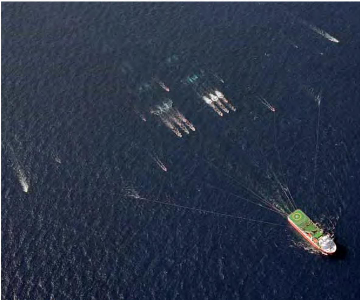
Seismic survey vessel for petroleum exploration. Photo: CCGVeritas.
