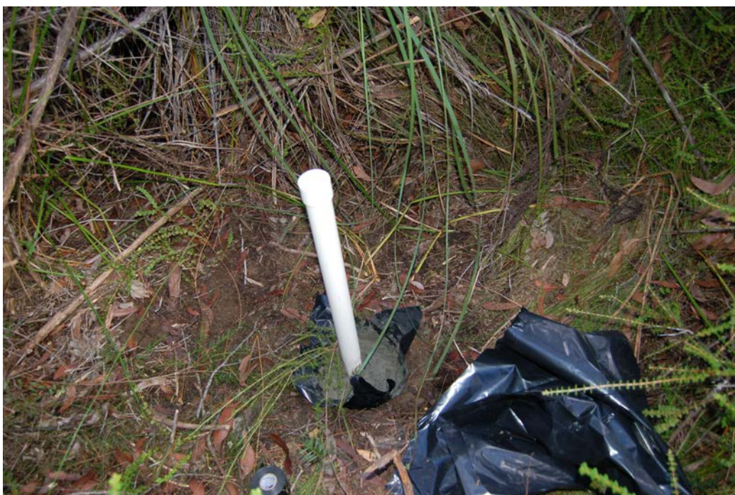
Figure 10: Piezometer used for sampling groundwater.
