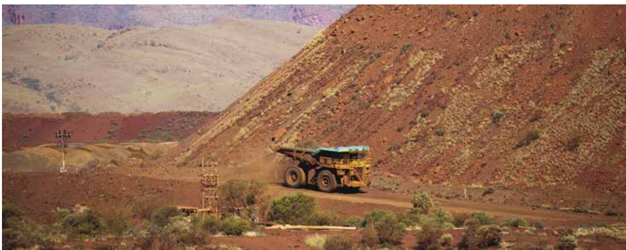
Iron ore mining requires the creation of huge waste dumps (as shown here) and the disposal of large volumes of water when mining drops below the watertable. Image: Krystle Wright
