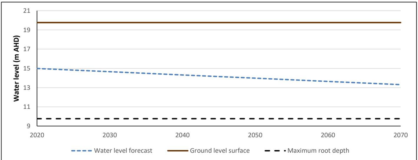
**Figure 4b.** A 50-year forecast of groundwater level decline at occurrences coolupbushland01 (46) and coolupbushland03 (47) (site ref: 61330068), calculated using the trendline ( $y = -0.0028x + 16.048$ ).
