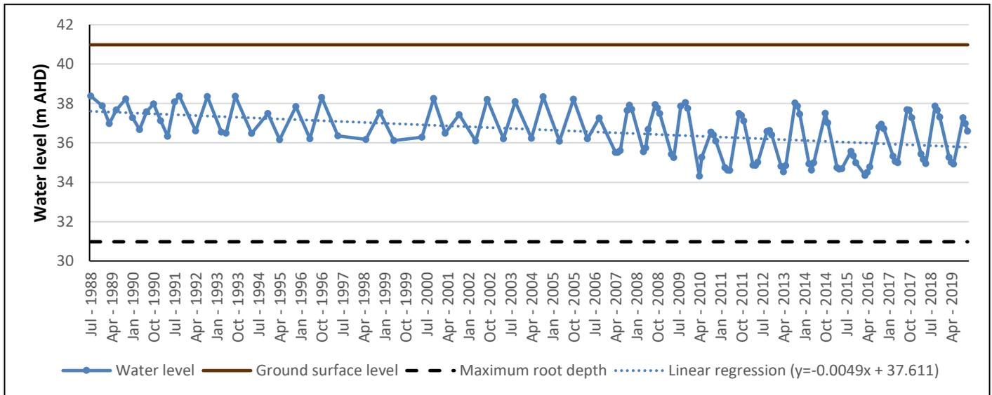
**Figure 3a.** Hydrograph of monitoring bore located 773m north of occurrence YARL01 (2) (site ref: 61330032), sampling the superficial Swan aquifer (DoW 2020).
