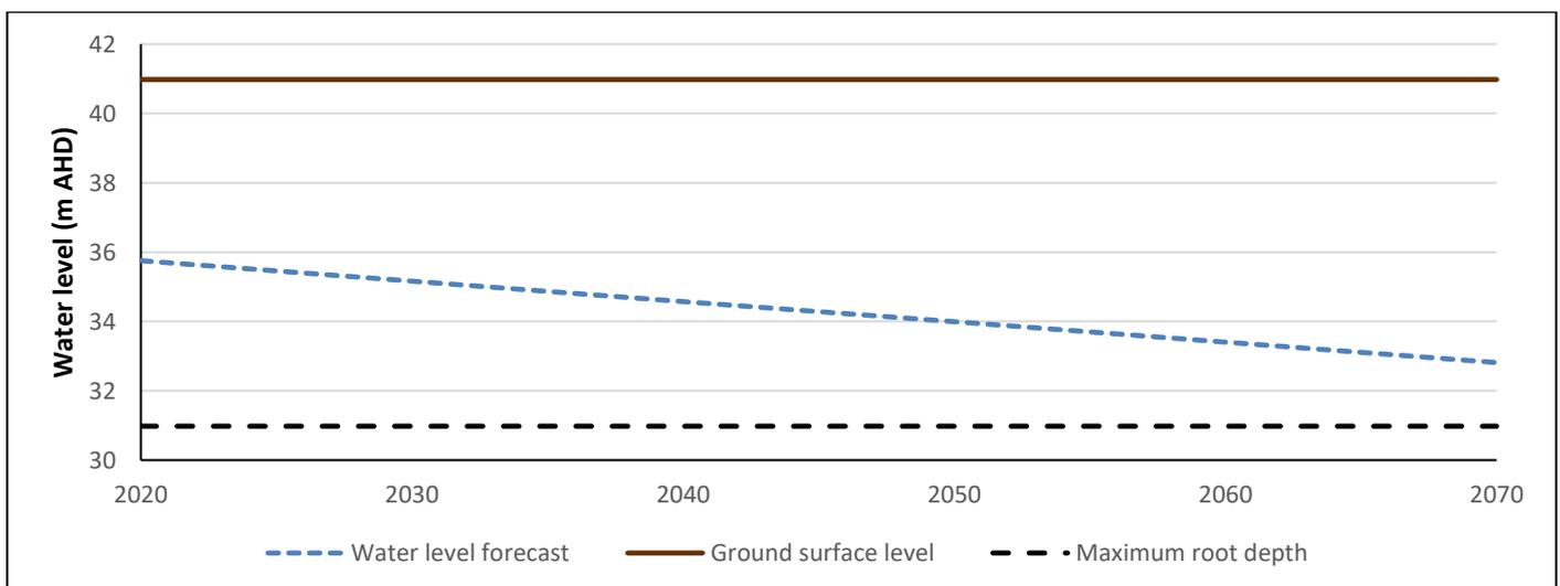
**Figure 3b.** A 50-year forecast of groundwater level decline at occurrence YARL01 (2) (site ref: 61330032), calculated using the trendline ( $y = -0.0049x + 37.611$ ).
