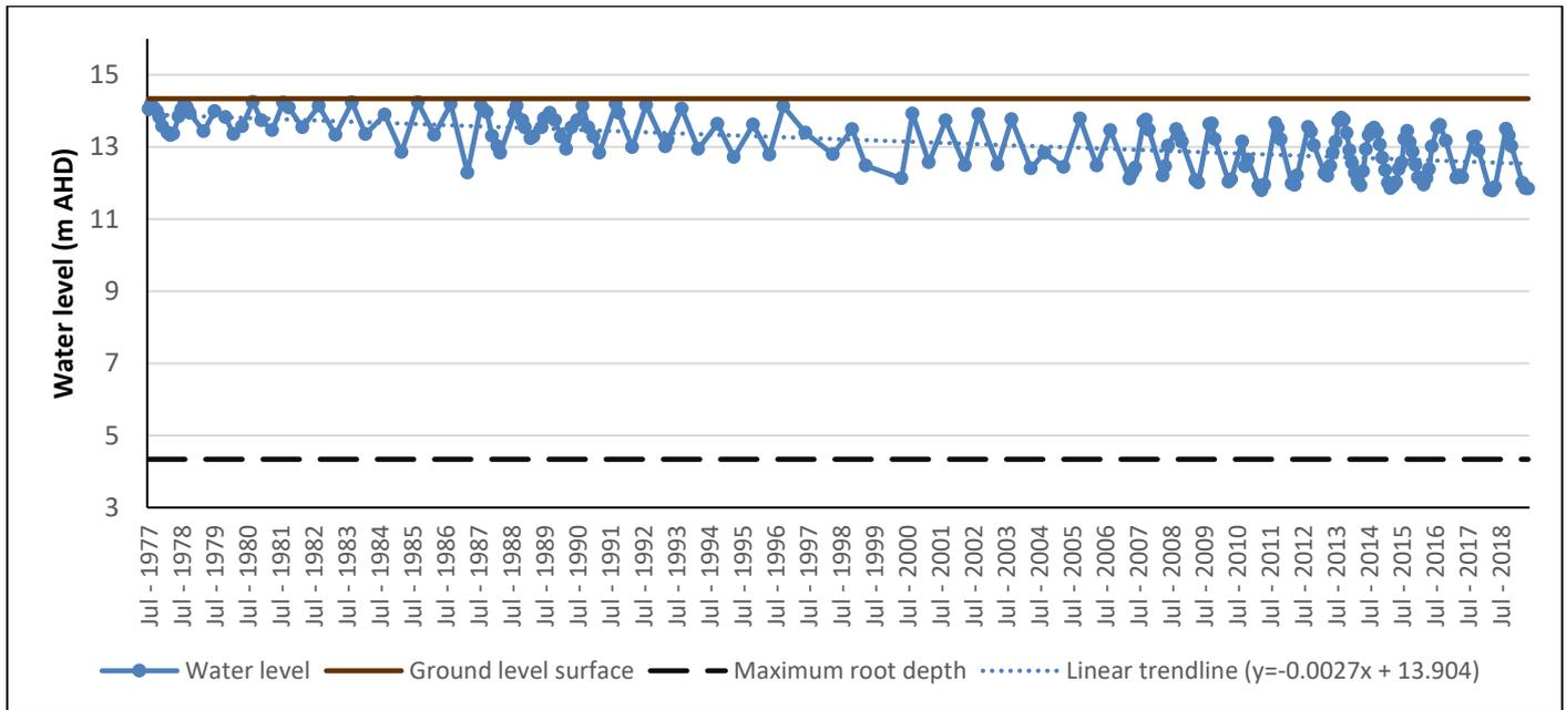
**Figure 6a.** Hydrograph of monitoring bore located 18m south of occurrence WATER03 (25), and 373m east of occurrence WATER06\_Webb (site ref: 61118038), sampling the superficial Swan aquifer (DoW 2020).
