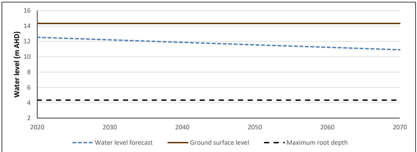
**Figure 6b.** A 50-year forecast of groundwater level decline at occurrence WATER03 (25) and WATER06\_Webb (40) (site ref: 61118038) calculated using the trendline ( $y = -0.0027x + 13.904$ ).
