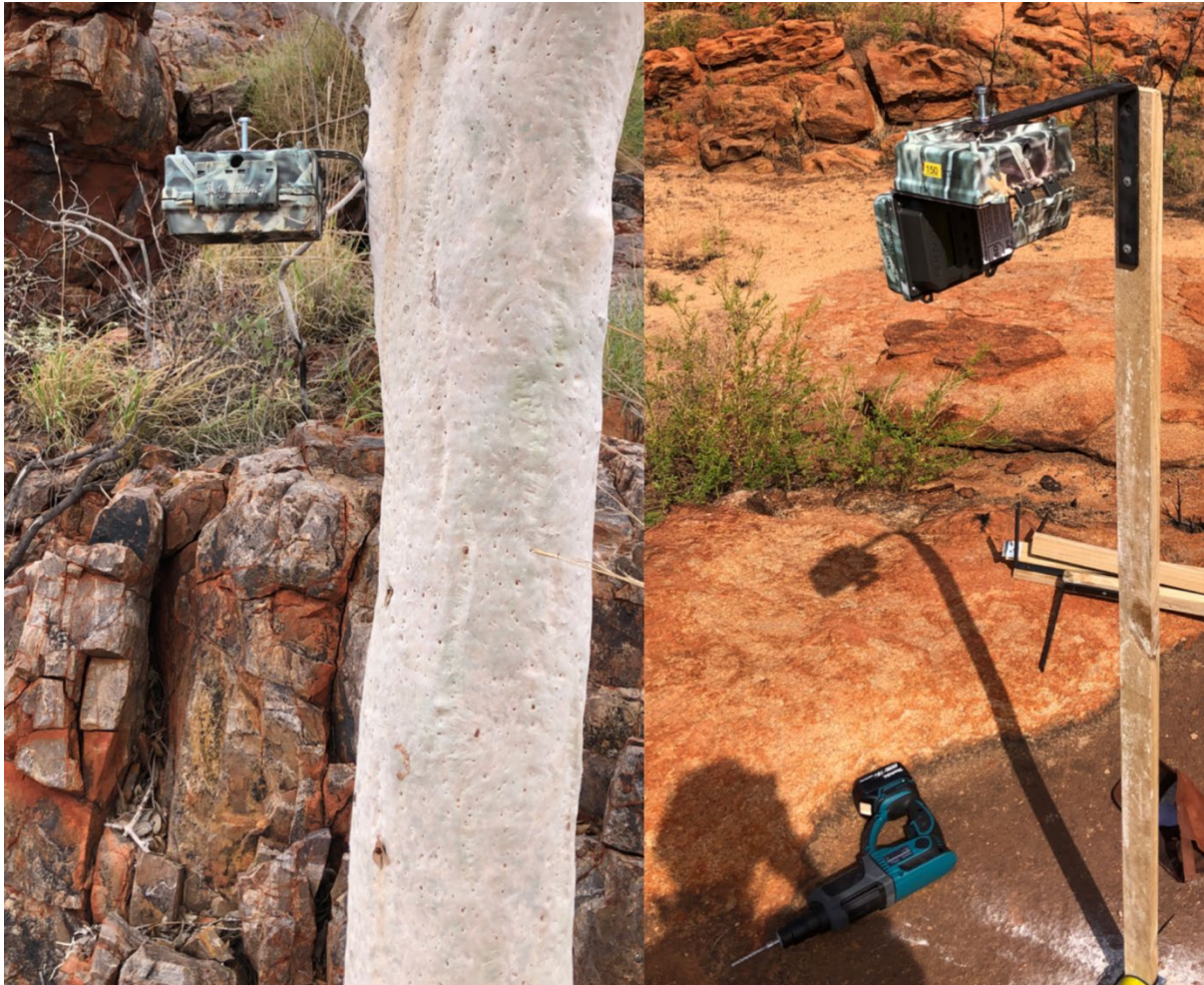
Figure 1.1-3 – Downward facing camera trap design used as part of the Pilbara northern quoll monitoring program. Cameras were mostly mounted to trees at a height of 1.5m. Where suitable trees were not available, wooden posts were bolted into the ground, and cameras were mounted to posts, following (Moore et al. 2021b).
