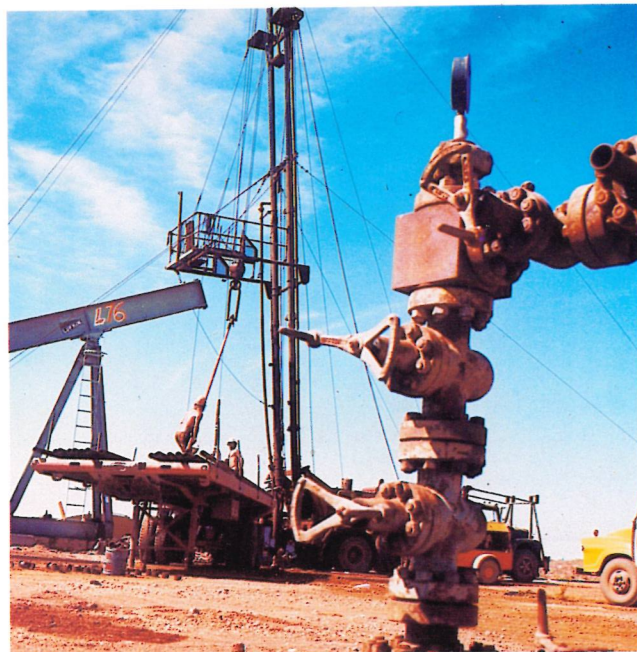
Workover rig on beam pump with "Christmas Tree" in foreground
