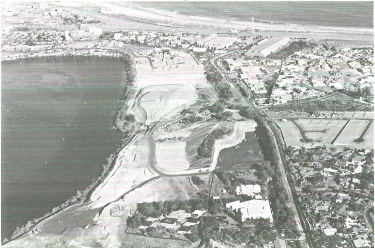
The Swan River foreshore adjacent to the McCabe Street redevelopment in Mosman Park is one example of a contaminated site in the Perth Region which is currently being cleaned-up. Upon completion of the clean-up program, the foreshore area will be covered with clean fill and rehabilitated to ensure that it is left in a stable condition. Photograph by Dr John Rogers.
