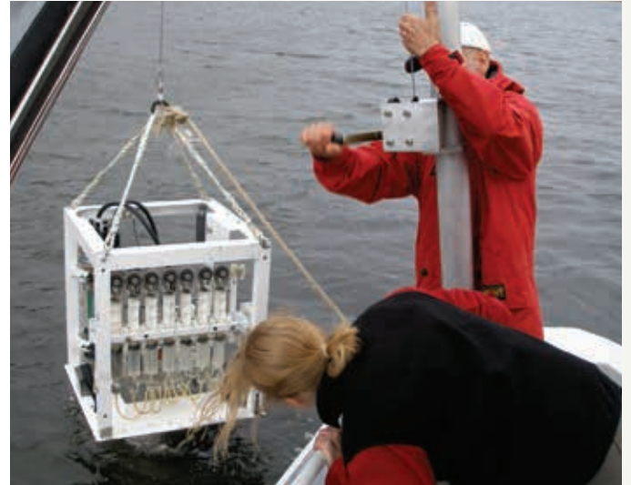
Deployment of a benthic chamber for investigating nutrient fluxes 2008. See also Figure 3.7. Courtesy Geoscience Australia and DoW.
