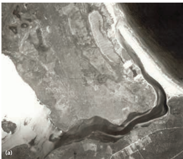
Figure 3.3 (a) Aerial Image of the Hardy Inlet entrance 1943. The passage through the bar is similar to that of the entrance in 2010. RAAF photograph #27738 Map 1136 Busselton-Karridale Run 2. After a channel on the western side of the bar was excavated in 1945 and floodwaters scoured a deep channel the position of remained in much the same location although is shallowed substantially and boat traffic to the ocean was at time difficult. By 1982 the entrance was moving eastwards as sand accumulated at Dukes Head and eroded from Point Frederick. (b) 2011 configuration of the inlet channel showing the similarity to 1943. Courtesy Brian Combley.
