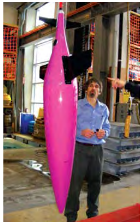
Fig 5 Slocum Glider: Ocean gliders are autonomous vehicles designed to operate in deep water and contain a suite of sensors to measure conductivity (for salinity), temperature, dissolved oxygen, fluorescence, turbidity, dissolved organic matter and down-welling light with depth. By changing its buoyancy, the glider is able to descend and ascend.
