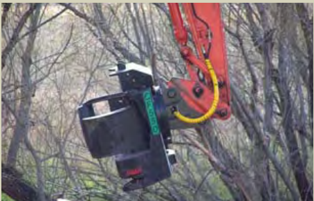
Specialised excavator heads can cut and apply herbicide in one action. (DPI Victoria)
