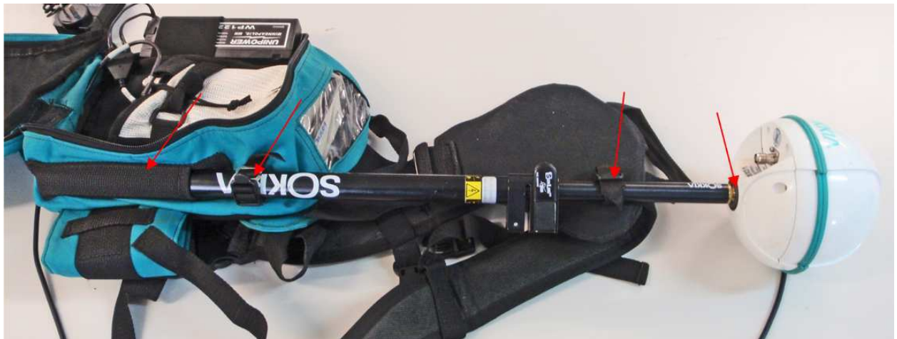
Figure 6. Placement of the antenna & pole onto the backpack. Note: red arrows indicate fastening points.
