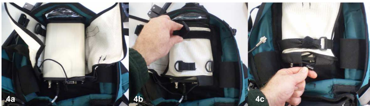
Figure 4a: Placement of the GIR 1400 Receiver into the backpack. Figure 4b: Fastening the velcro strap around the receiver. Figure 4c: Tightening the drawstring at the base of the receiver.
