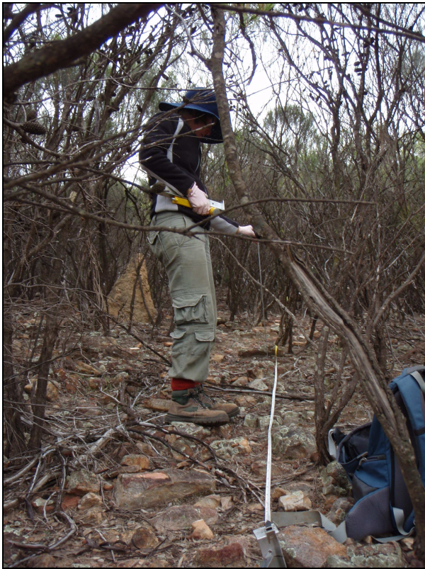
Plate 1 Using a point intercept device to record species intercepting the transect line.
