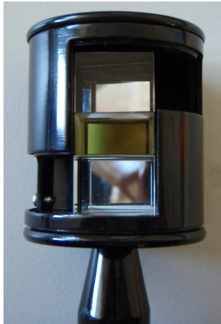
Figure 2 Optical Square showing three prisms
