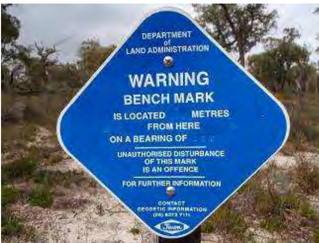
Photo 9: 'Landgate' Witness Plate at Goonaping Swamp in Sep 2008.
