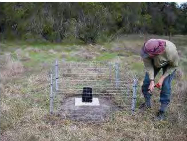
Photo 28: Tipping bucket rainfall recorders have been installed on 14 wetlands. Alan Clarke, 17Jun2009.
