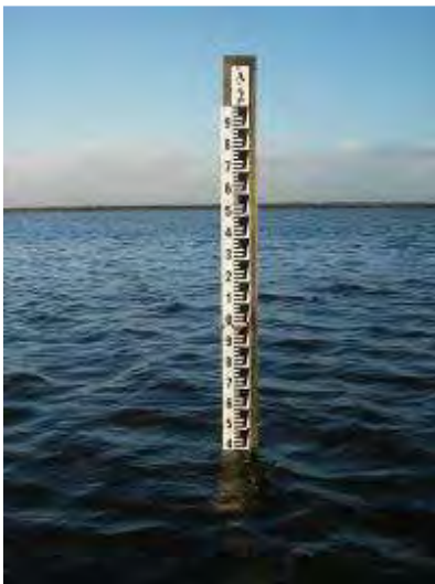
Photo 4: DPaW depth gauge 'A' at Parkeyerring Lake on 18Jul2008 read 0.40m.
