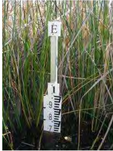
Photo 2: DPaW depth gauge 'E' at Thomsons Lake on 04Aug2008 read 0.70m.
