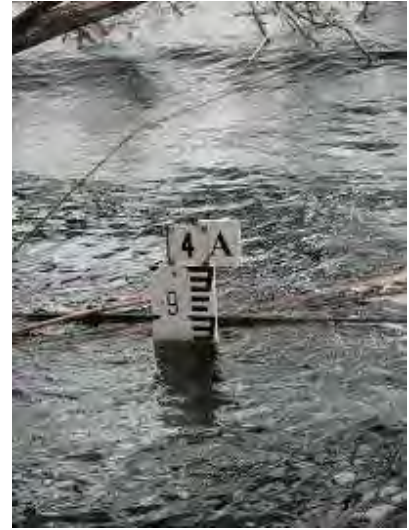
Photo 3: DPaW depth gauge 'A' at Lake Wilson on 03Nov2008 read 3.85m.
