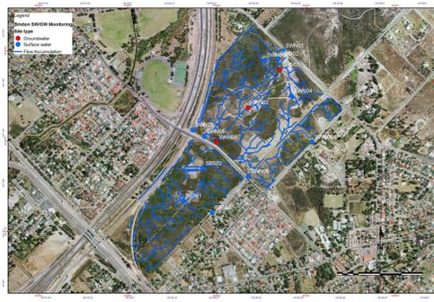
Figure 3. DBCA monitoring infrastructure and watershed generation analysis for the Brixton Street Nature Reserve and Wanaping Block.
