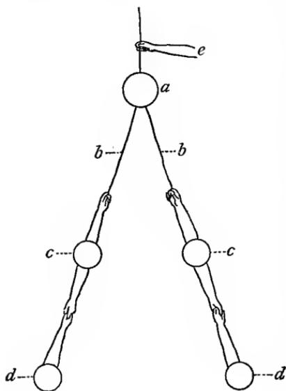
figure) was passed through the phial (*a*), the two ends of which were taken hold of by two people (*c c*), who each took hold of another person (*d d*); the operator (*e*) then touched the phial with his discharging wire, and received the shock through both arms, as did (*c c*) and (*d d*). Sometimes, however, the others (*d d*) felt it only in the arm by which they held (*c c*). The comparative force of the blows which each felt were difficult to ascertain, but we supposed that (*c c*)
