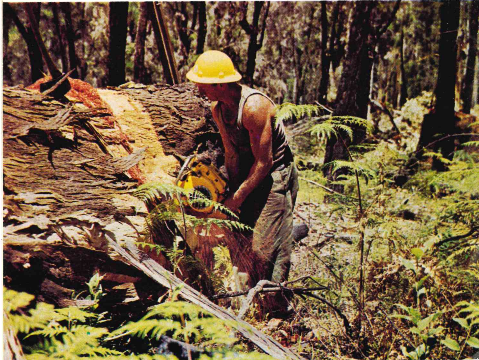
Chain sawing a log into suitable lengths for hauling.
