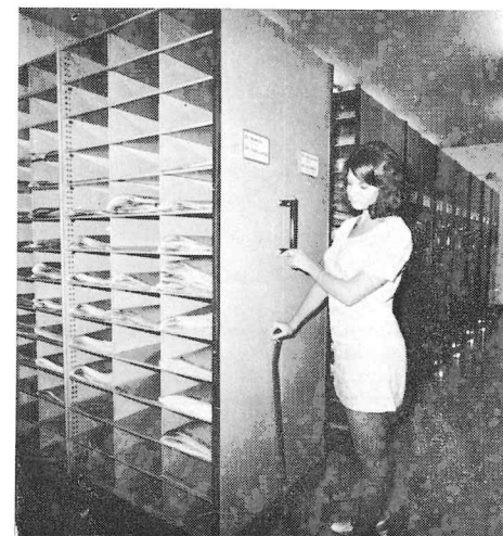
"Compactus" cupboards in which the herbarium specimens are stored are powered by an electric motor for easy movement.
