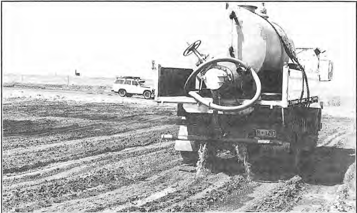
Figure 1: Karratha land application site. Oil contaminated water is applied here using the vehicle's own boom-spray. This method has since been modified by using an offset boom-spray towed behind the vehicle to avoid splash-back and bogging. The bund walls and fencing prevent unlawful dumping and aid in flood control.
