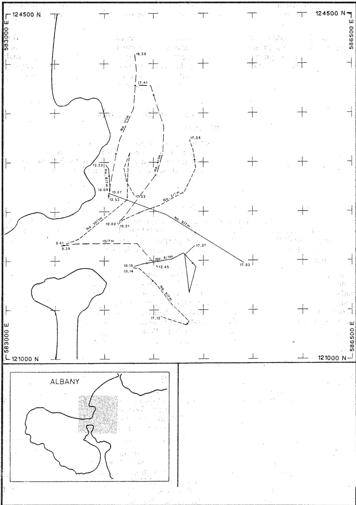
Figure 31: Drogue trajectories in King George Sound induced by ebb tide and south-south-east wind; 15 August 1985, 0930 to 1754.
