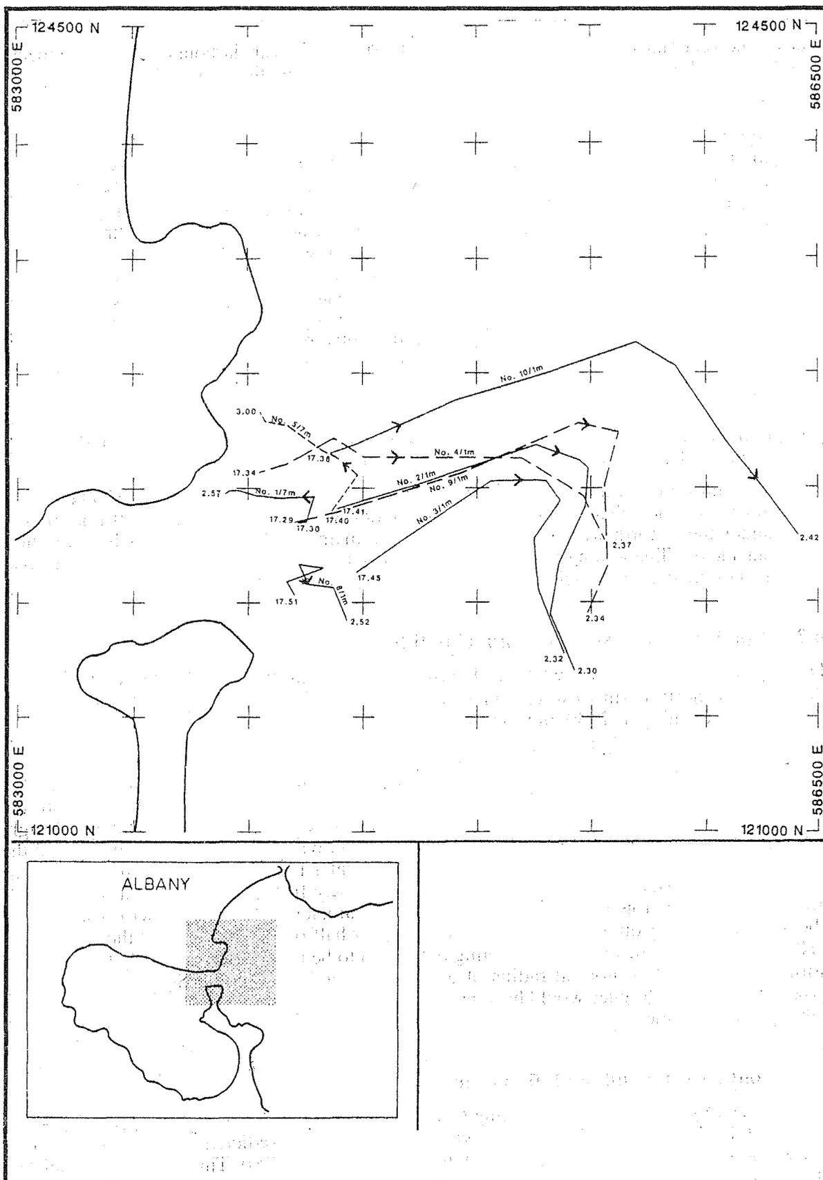
Figure 32: Drogue trajectories in King George Sound for early flood tide and north-west winds; 27-28 August 1985, 1730 to 0300.
