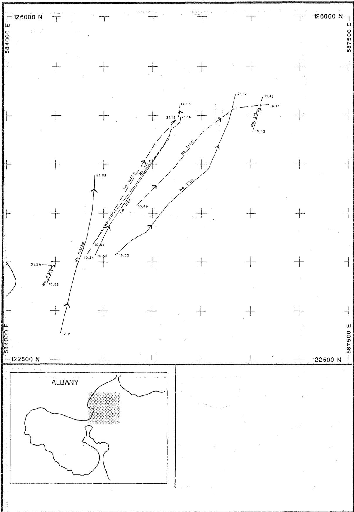
Figure 34: Drogue trajectories in King George Sound of flood tide and north-north-west winds; 23 February 1986, 1040 to 2116
