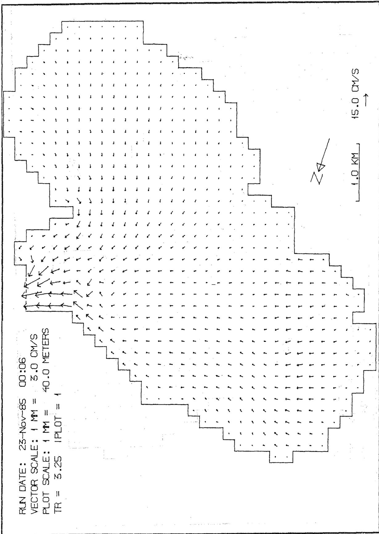
Figure 8: Modelled, instantaneous water current distribution in Princess Royal Harbour, subject to a diurnal tide of range 1m; time of Low Water + 18 hours.
