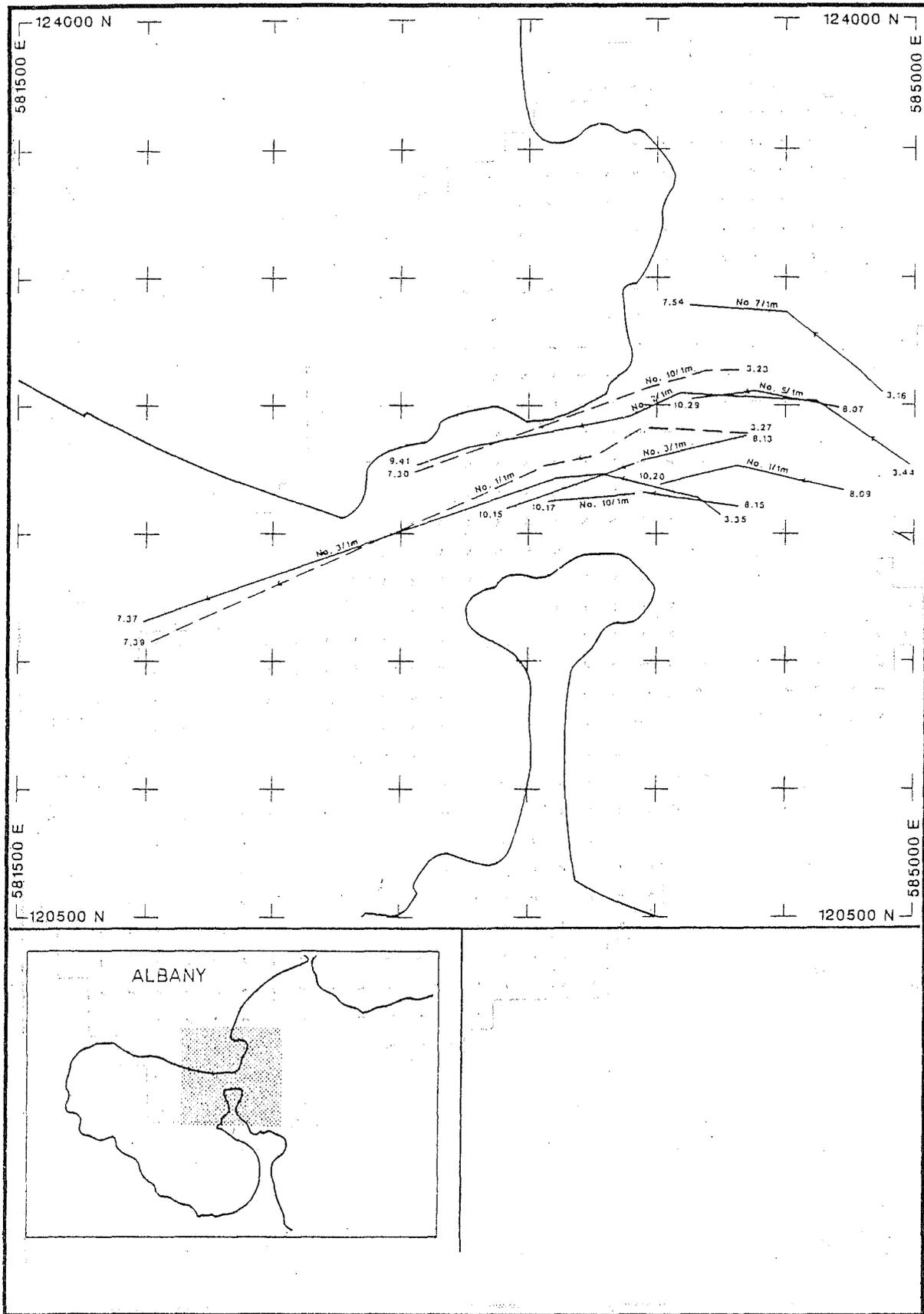
Figure 12: Drogue trajectories in King George Sound released within 1km of the Princess Royal Harbour entrance during a flood tide and light wind conditions on 23 May 1985, 0316-1017
