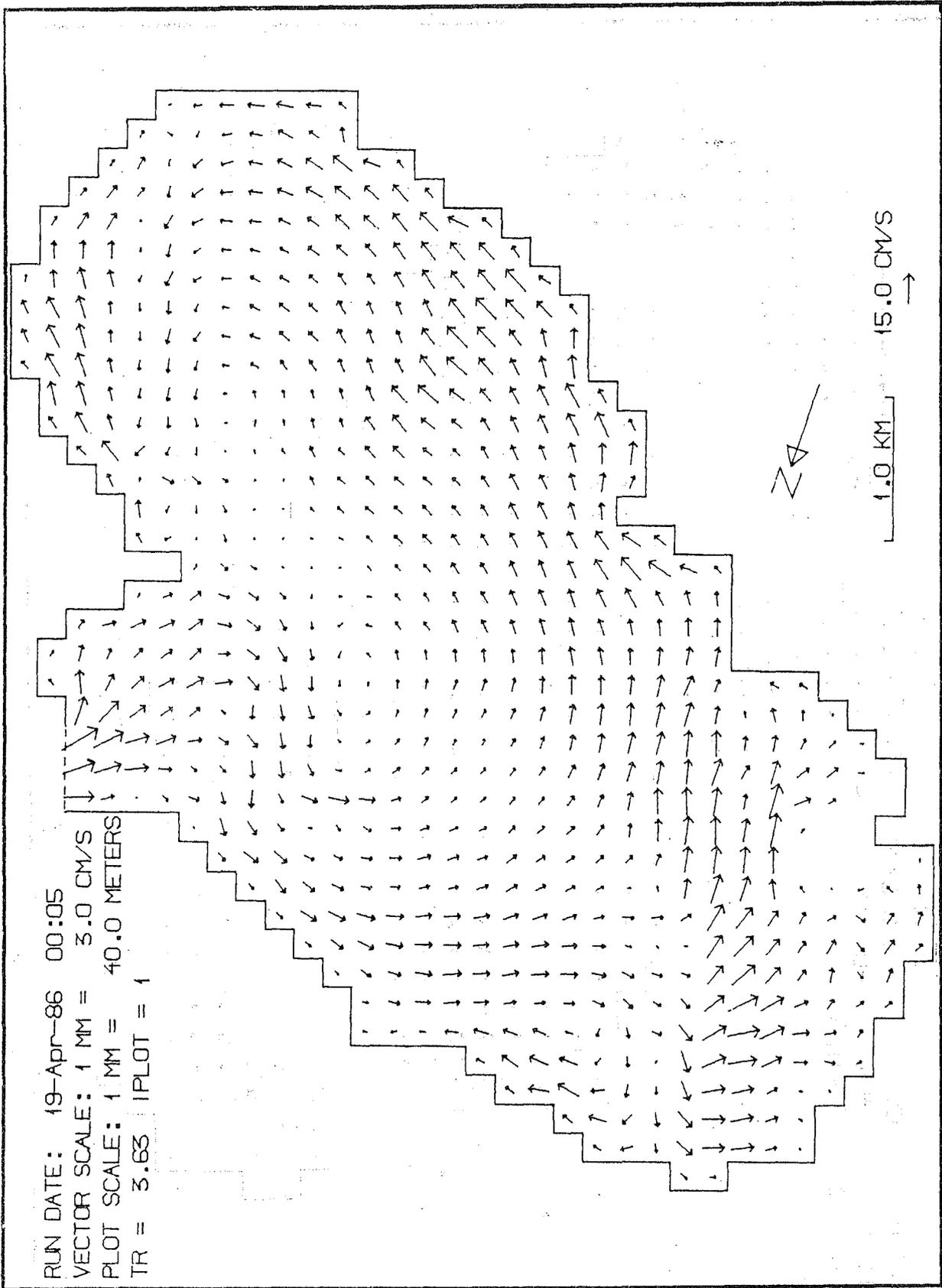
Figure 14: Modelled, instantaneous water current distribution in Princess Royal Harbour, subject to a diurnal tide of range 1m and northwest wind of  $7.5 \text{ ms}^{-1}$ ; time of Low Water + 3 hours.
