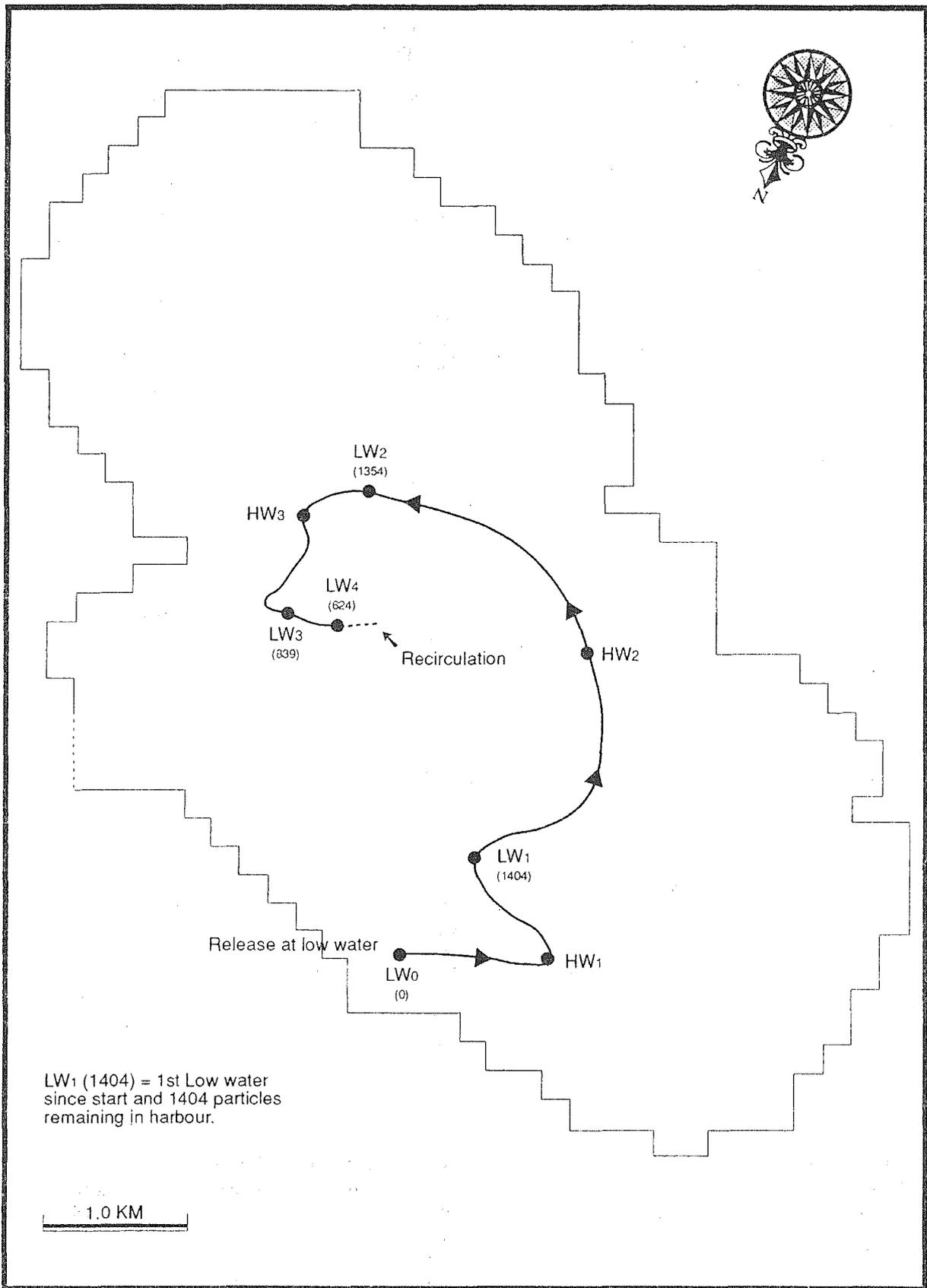
Figure 25: Modelled trajectory of the centre of mass of effluent released in Princess Royal Harbour (from source 2) for a diurnal spring tide of range 1m and north-west wind of 7.5ms<sup>-1</sup>
