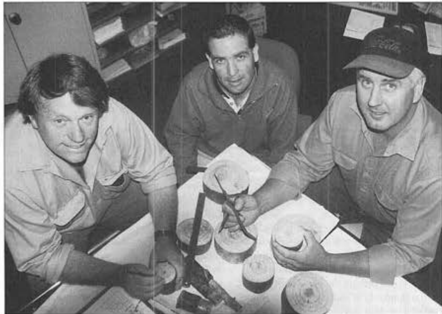
Terry Carpena, Andrew Rumley and John Terry use calipers and magnifying glasses to count the growth rings from plot bluegums. Photo by Jo Wallace.
