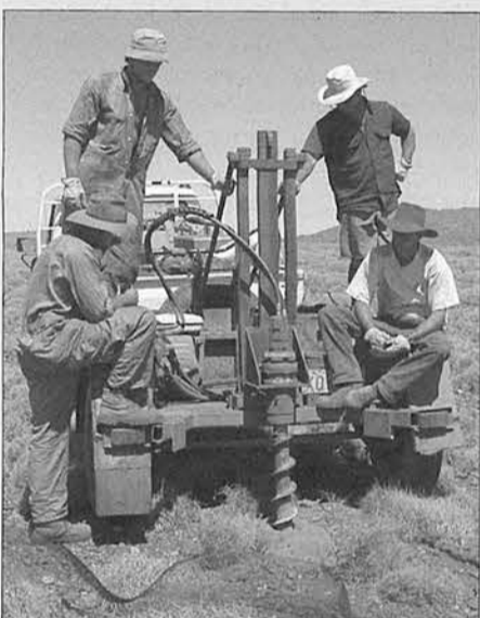
Staff members (from left) Patrick Cullen, Tristan Farmer, Dan Kamien and Roger Whitelaw use their weight to assist a mobile drilling rig to drill holes for vertebrate pit traps in the hard Pilbara landscape. The traps catch small ground dwelling creatures such as dunnarts, skinks, geckos and small dragons. Photo – Jim Rolfe
