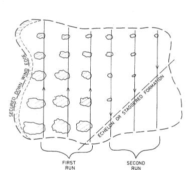
Strips are started on the downwind edge of the burn and move progressively up wind. Hatching illustrates area burnt.
