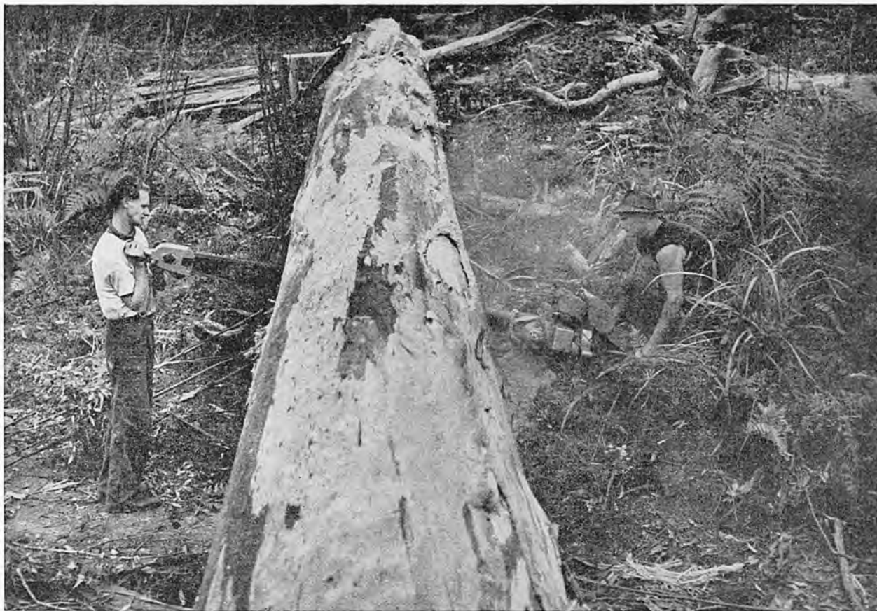
Plate 18. Crosscutting a large karri log with a power chain saw.
