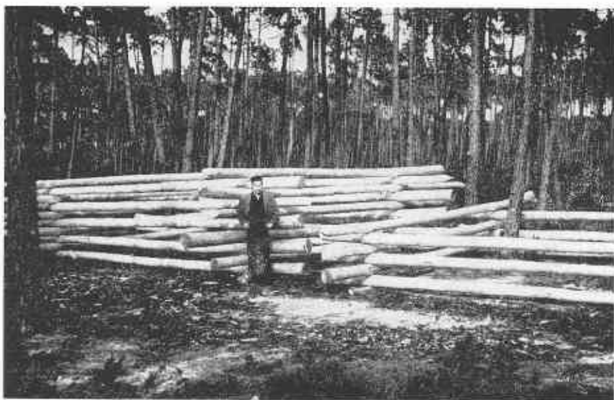
Figure 17.— Pinus pinaster poles for the Post Office Department. Air seasoning prior to Tanalith treatment.
