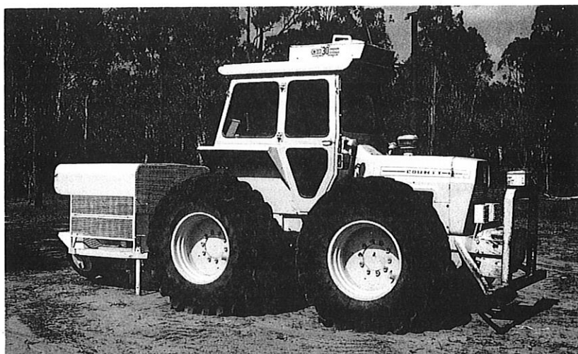
Figure 3: Tractor and planting machine. County tractors are favoured in Queensland because of better efficiency attributed to the true four-wheel drive design.
