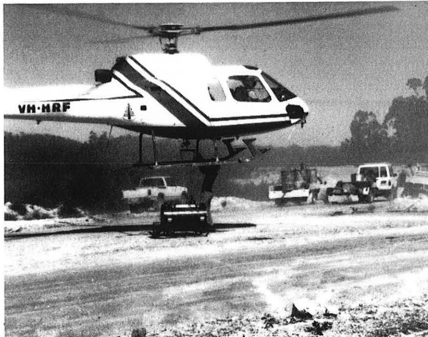
FIGURE 6. LIFTING STRAP BEING HOOKED TO HELICOPTER
