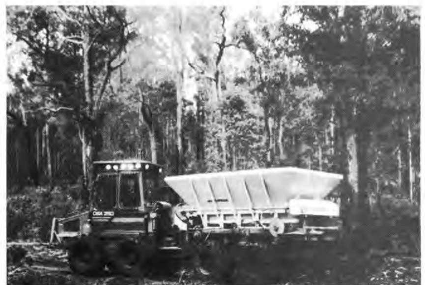
A gypsum spreader is attached to a forwarder to spread fertiliser in pine plantations.
