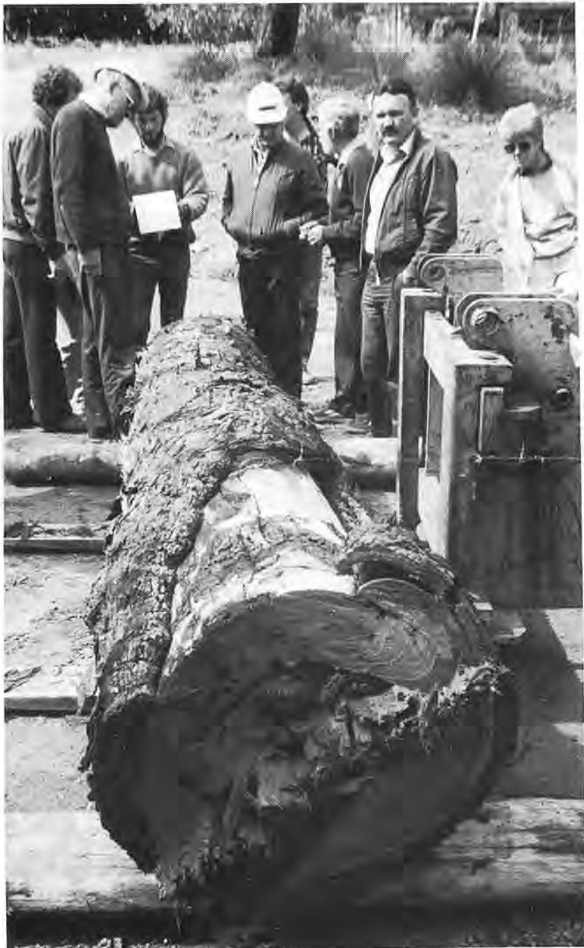
CALM staff examine the exterior of a jarrah log before it is sawn, to determine its defects.
