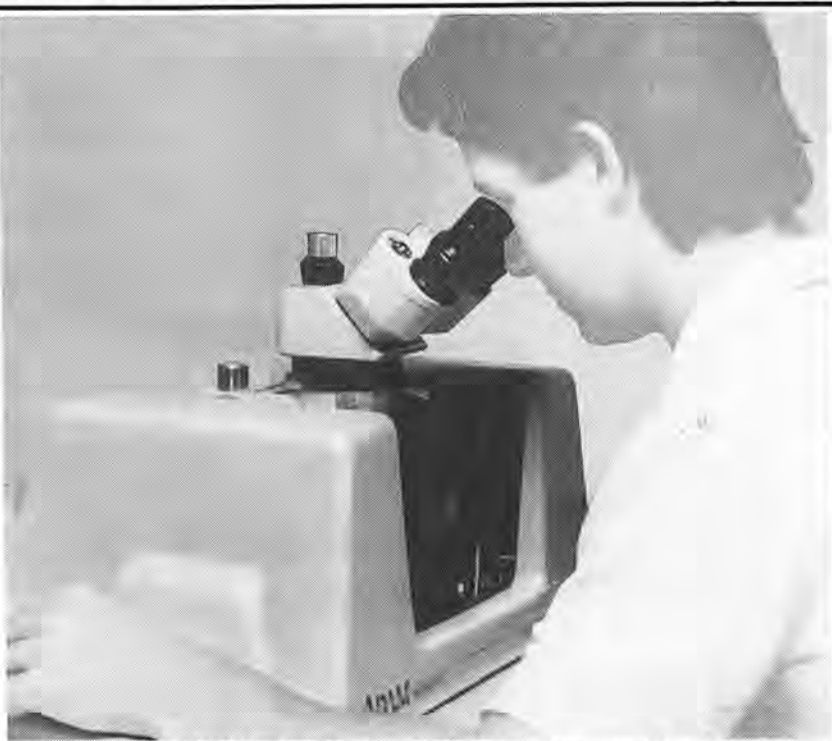
CARTOGRAPHIC Draftsman Mark Laming uses the MPS2 to calculate the volume of woodchips in a pile. The entire system weighs only 10kg, making it easily portable.
