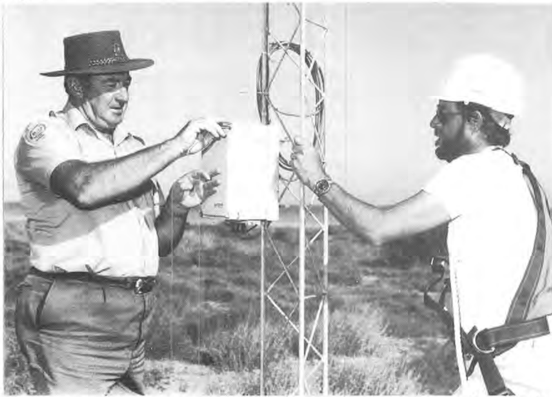
Mobile Ranger Barry Cartledge (left) changes the data logger at the Ningaloo meteorological station, while Ian Parker prepares to climb up to install a repaired instrument head.
