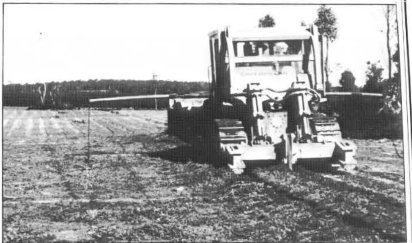
A D7 dozer rips to a depth of 60 cms, the marker chains on the sides determine the distance a part of the line and its return run.
