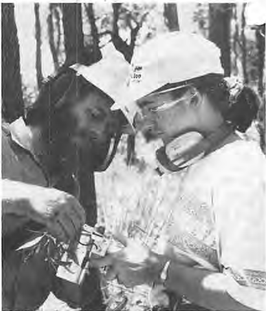
Technical officer Rick Giles helps volunteer Helen Williams measure transpiration of jarrah leaves with a porometer.
