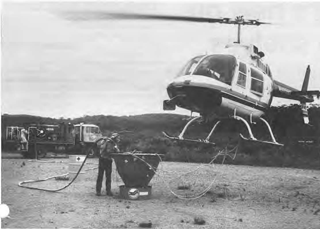
A helicopter fitted with a 'monsoon' bucket can make a significant difference in bringing a fire under control and keeping it that way. Filling the bucket prior to take-off is Manjimup forest ranger Leon Price. Meanwhile, back at the truck is fire equipment officer Gary Kravainis of Fire Protection Branch. See 'Helicopter buckets fire at Walpole-Nornalup NP' on page 4. Photo by Lachlan McCaw
