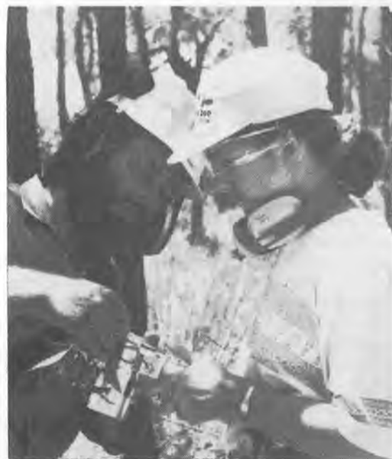
January — Technical officer Rick Giles helps volunteer Helen Williams measure transpiration of jarrah leaves with a porometer. Photo by Barb Giles
