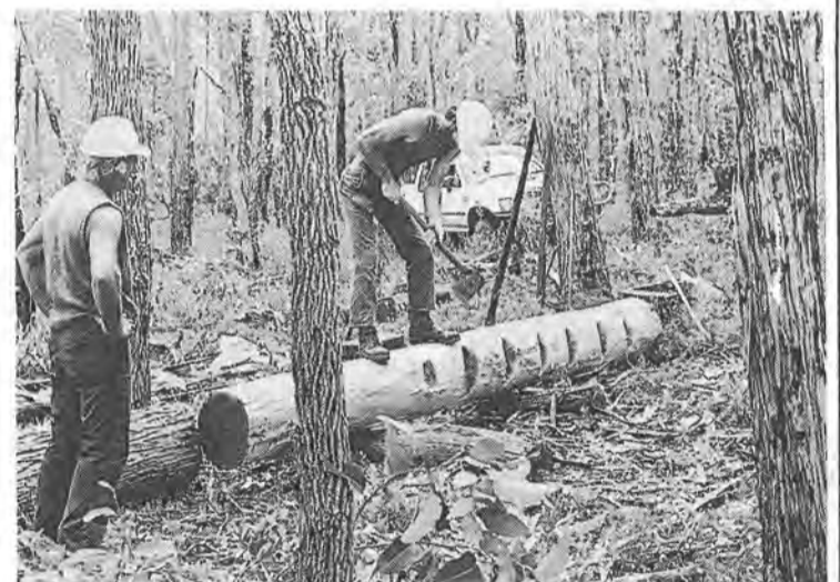
Preparing to flat the edge before hollowing. Peter Rado, left, offers guidance to Steve Winfield.
