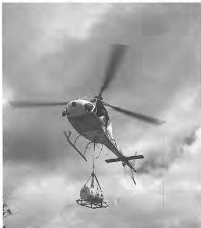
A helitorch suspended below the helicopter used in the prescribed burning program. Photo by Tammie Reid
