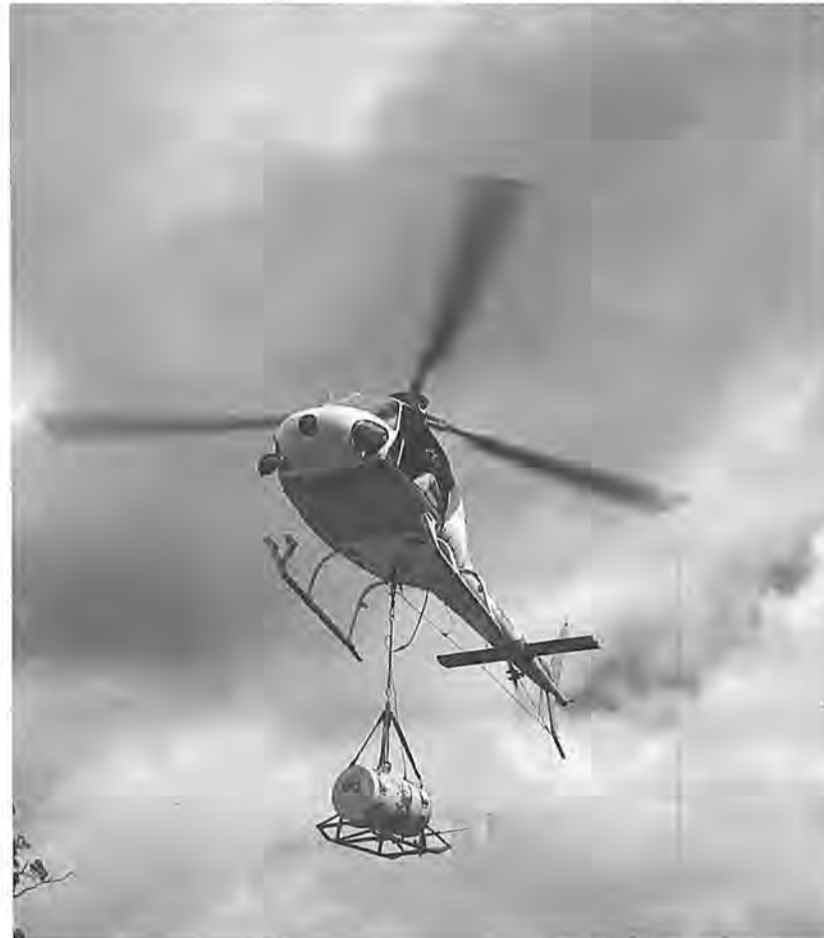
A helitorch suspended below the helicopter used in the prescribed burning program. Photo by Tammie Reid
