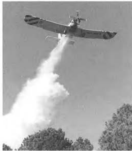
The key to Operation Firebird is the Dromader M-18A, seen here dropping 3000 litres of foam-water mix. Photo by Norm Bailey
