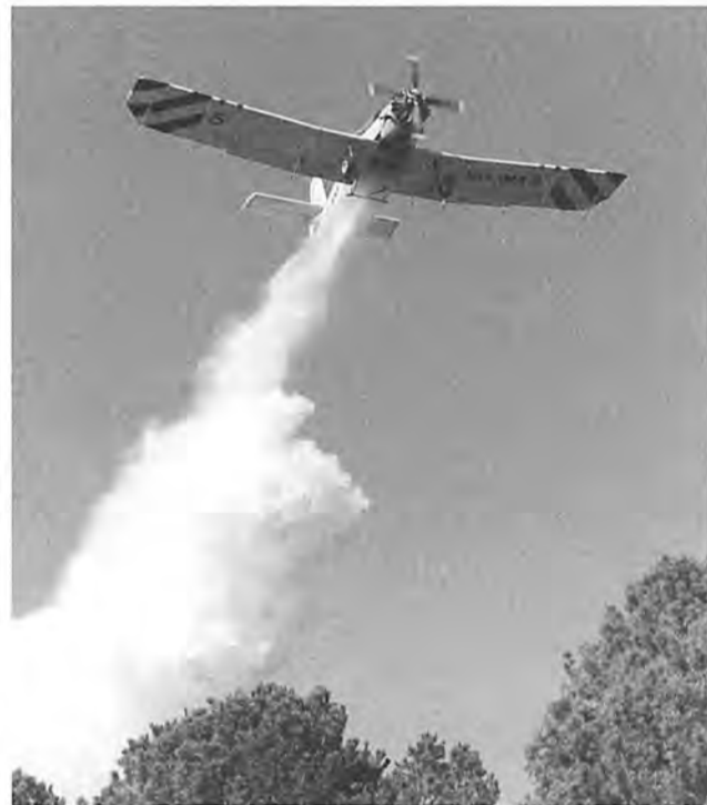
The key to Operation Firebird is the Dromader M-18A, seen here dropping 3000 litres of foam-water mix.
