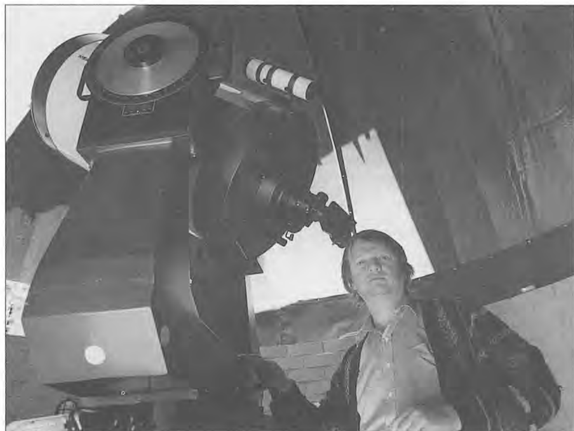
CALM's Perth Observatory technical manager Arie Verveer was responsible for the management and much of the logistics involved in the erection of a new building (officially opened in August) to house this Meade 40-cm aperture Schmidt-Cassegrain telescope. At present this telescope is mainly used by the public to view faint celestial objects during the Observatory's very popular star-viewing nights. Photo by Ernie McLintock
