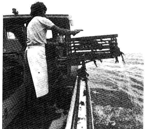
Pot tippers and winches are used to haul in and bring the heavily weighted pots aboard.
