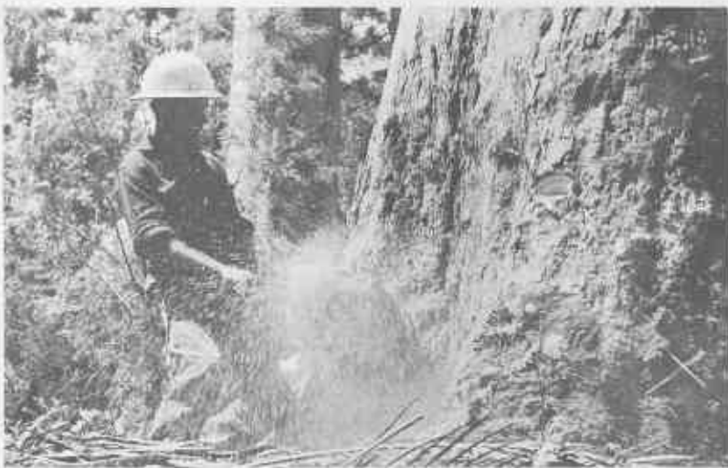
Commencing the "backing down" cut
