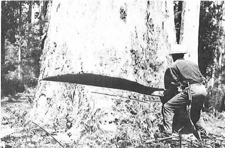
Karri felling sequence: Feller removes wedge of wood from scarf
