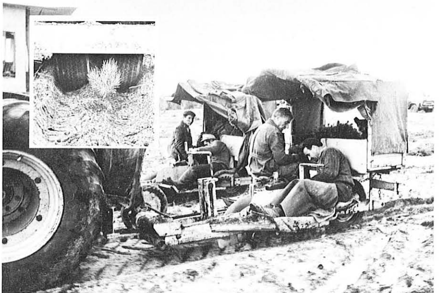
Tandem planting machine in operation on coastal sands north of Yanchep. Inset shows seedling emerging from the tamping wheels.
